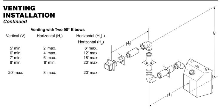
Figure 19 - Horizontal Termination Configuration for Rigid Venting Using Two 90° Elbows
